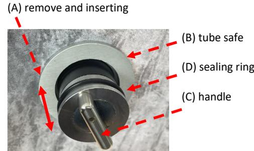
**Lock and unlock the keysafe**
